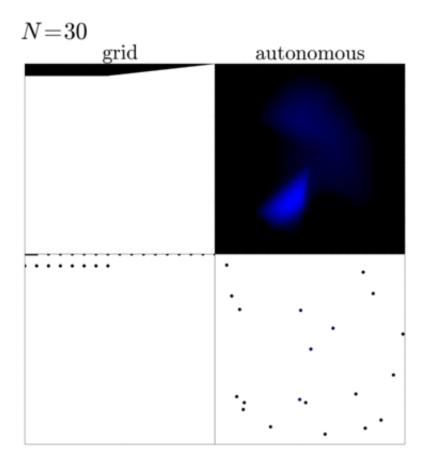
This animation shows a comparison between a traditional grid measurement (left) of a sample with a measurement steered by the newly-developed decisionmaking algorithm (right). This comparison shows that the algorithm can identify the edges and inner part of the sample and focuses the measurement in these regions to gain more knowledge about the sample. Credit: Brookhaven National Laboratory
