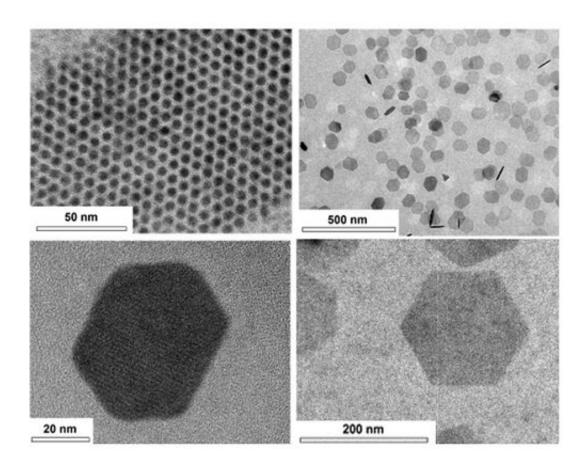
Uniformly ordered single-crystalline graphene quantum dots of various sizes synthesized through solution chemistry. Credit: KAIST
