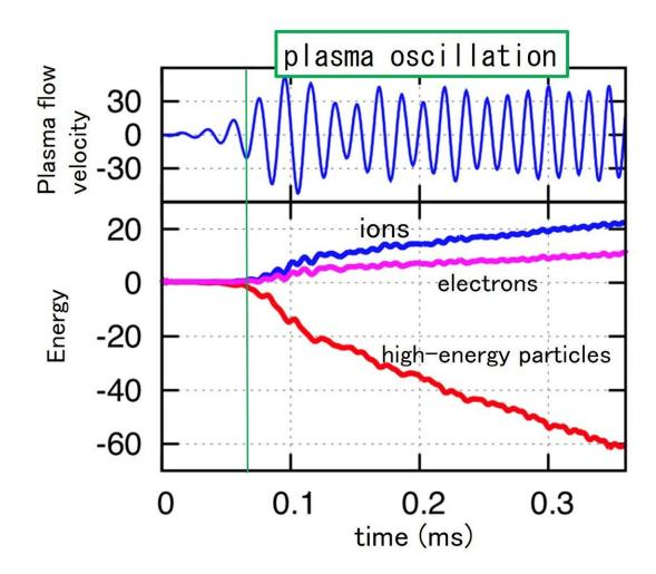
Time variations of plasma oscillation and energy of ions, electrons, and highenergy particles. Credit: NIFS
