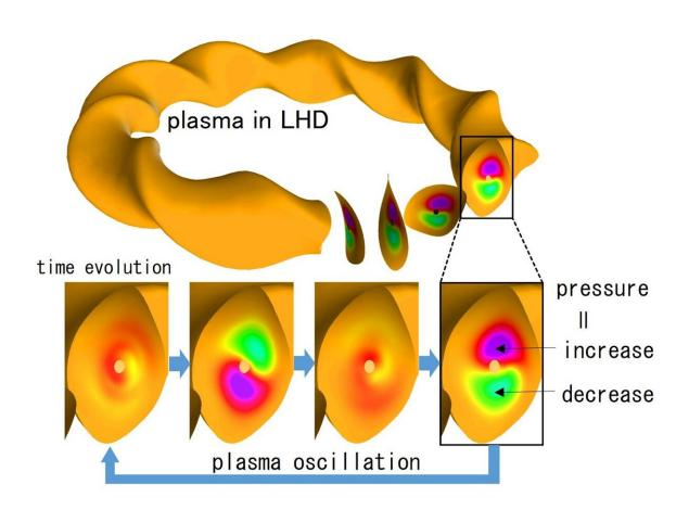
Plasma oscillations driven by high-energy particles in a plasma in LHD. Credit: NIFS
