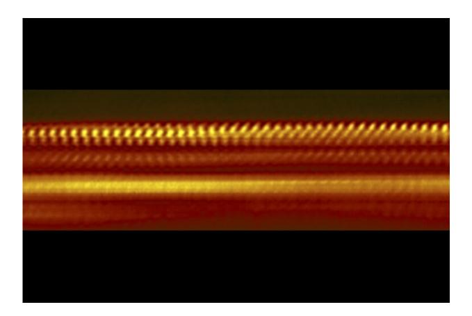
This greatly magnified image shows four layers of atomically thin materials that form a heat-shield just two to three nanometers thick, or roughly 50,000 times thinner than a sheet of paper. Credit: National Institute of Standards and Technology
