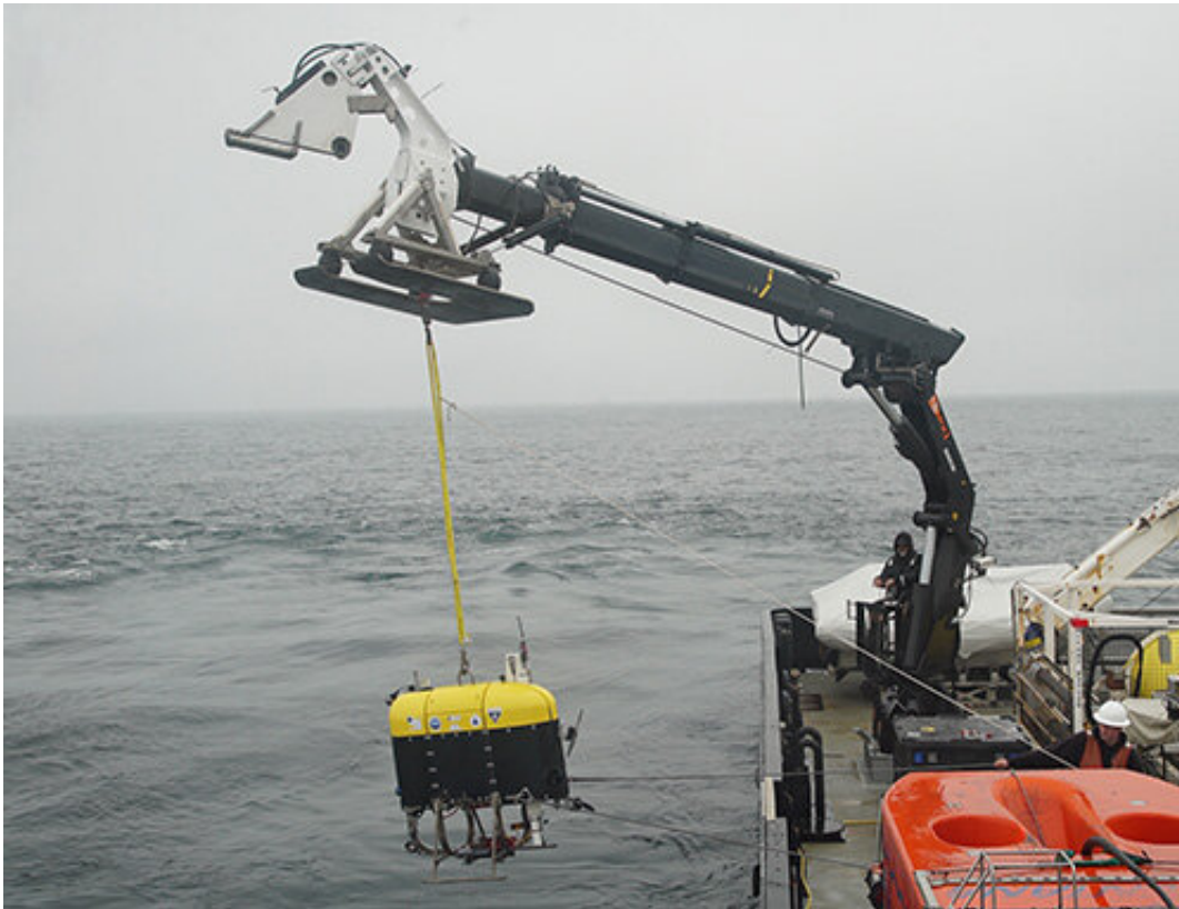
Launching the Mesobot from the deck of MBARI's research vessel Rachel Carson. Credit: WHOI/ Erik Olsen
