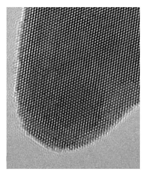
An image from an electron microscope shows the arrangement of the atoms on the gold nanosheet. Credit: University of Leeds
