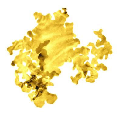
A gold nanosheet that is just two atoms thick. It has been artificially coloured. Credit: University of Leeds
