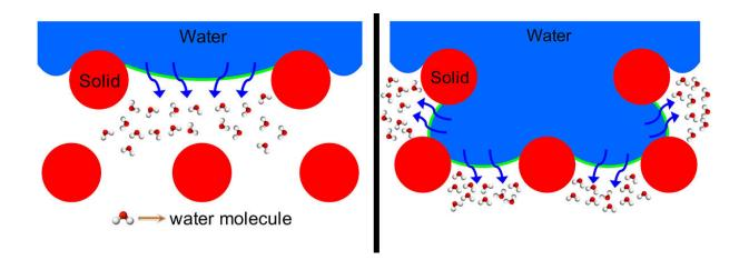
Left represents an omniphobic membrane, and right represents a conventional hydrophobic membrane with increased water-air interfacial areas (green lines). Credit: Kota lab
