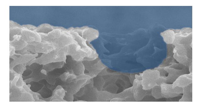
Cross-sectional view of a conventional hydrophobic membrane used in membrane distillation. The blue represents water. Credit: Tong and Kota labs
