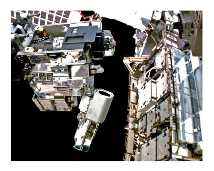
Robotic Refueling Mission 3's Multi-Function Tool 2, operated by Dextre, demonstrates robotic refueling operations on the outside of space station. Credit: NASA
