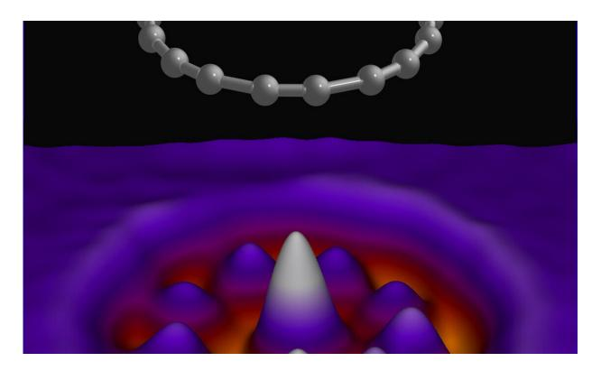
Cyclo[18]carbon. Bottom: artistic 3-dimensional representation of AFM data (at increased tipsample distance); top: molecular structure model. Credit: IBM Research
