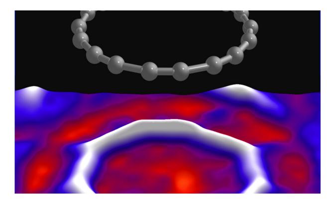
Cyclo[18]carbon. Bottom: artistic 3-dimensional representation of AFM data (at small tipsample distance); top: molecular structure model. Credit: IBM Research
