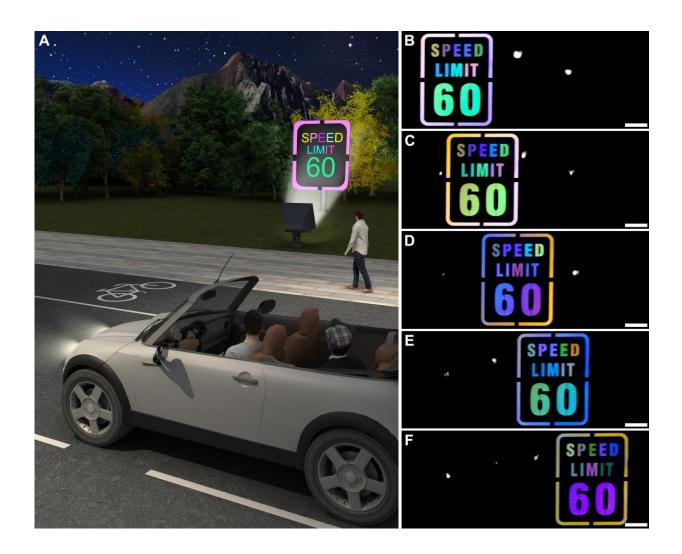
An image series shows how a new retroreflective material can be used to make a color-changing speed limit sign. Boxes A-F show how the sign changes color, from the perspective of drivers on the road, as they pass by. Credit: Fan et al., *Sci. Adv.* 2019; 5 : eaaw8755. CC BY-NC
