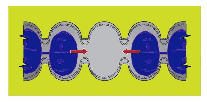
To squeeze a particular cavity cell, balloons are placed inside the cells surrounding it. The balloons support these cells, resulting in the unoccupied cell being reshaped as forces are applied to each end of the cavity. Credit: Diana Brandonisio
