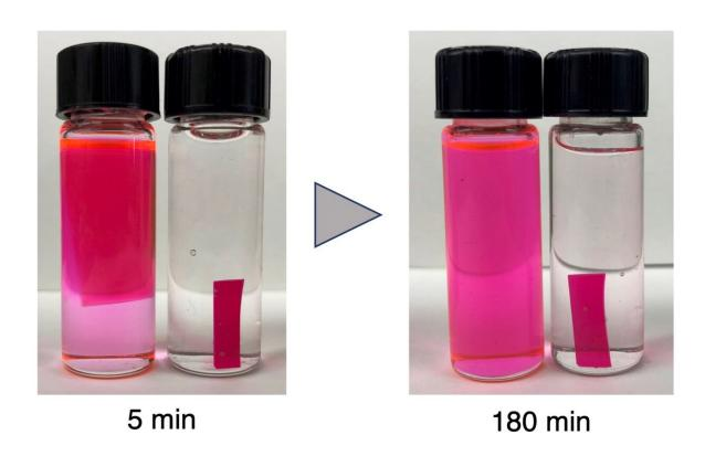
The degradable polyurethane material (pink strip) swells and then dissolves in acid mixed with an organic solvent (left vial in both photos) but not when placed in acid mixed with water (right vial in both photos). Credit: Steven Zimmerman and Ephraim Morado
