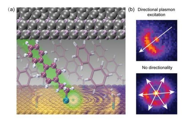
Figure (a) shows an artistic impression of the directional tunnelling in a molecular double-barrier junction followed by plasmon excitation [Credit: Harshini Venkata ANNADATA]. Figure (b) gives the experimental defocused light emission images showing the directional excitation of surface plasmon polaritons for samples containing molecules with and without a specific tilt angle. Credit: Nano Letters
