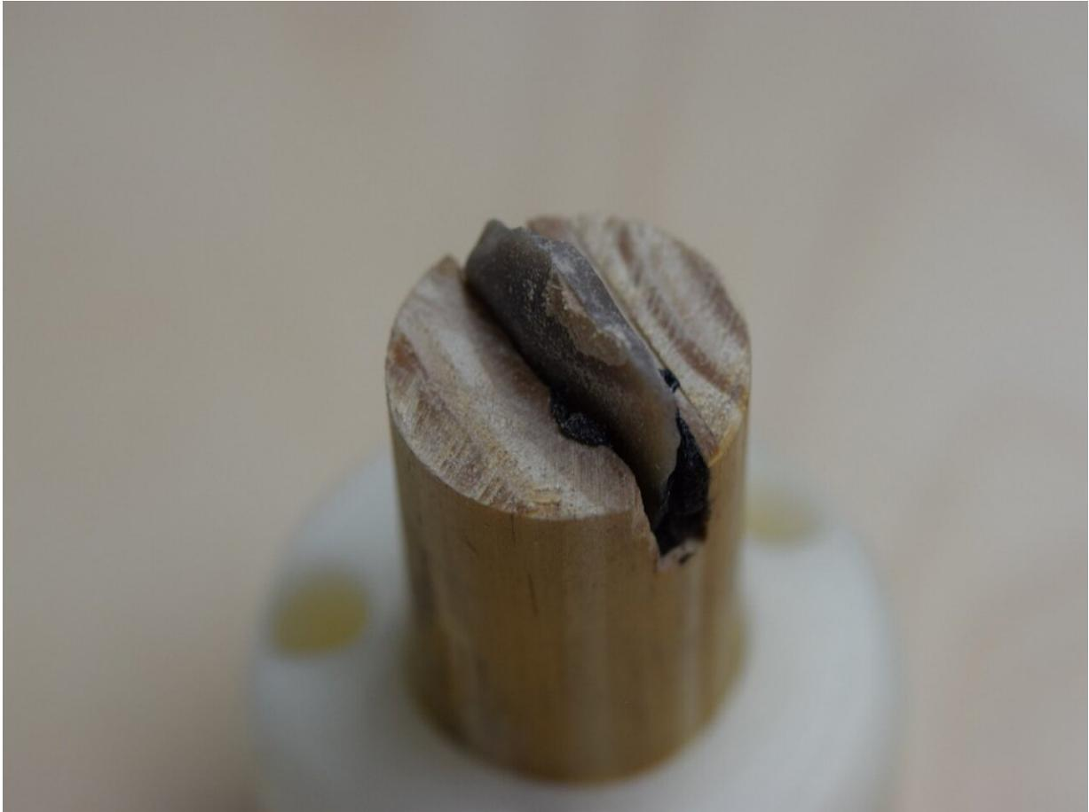
Researchers used birch pitch to attach flint to wood, as Neanderthals would have done, but the wood was fashioned into a type of drill bit so their force-controlled robotic arm could precisely test the adhesion. Credit: NYU Tandon, Johannes Pflieger
