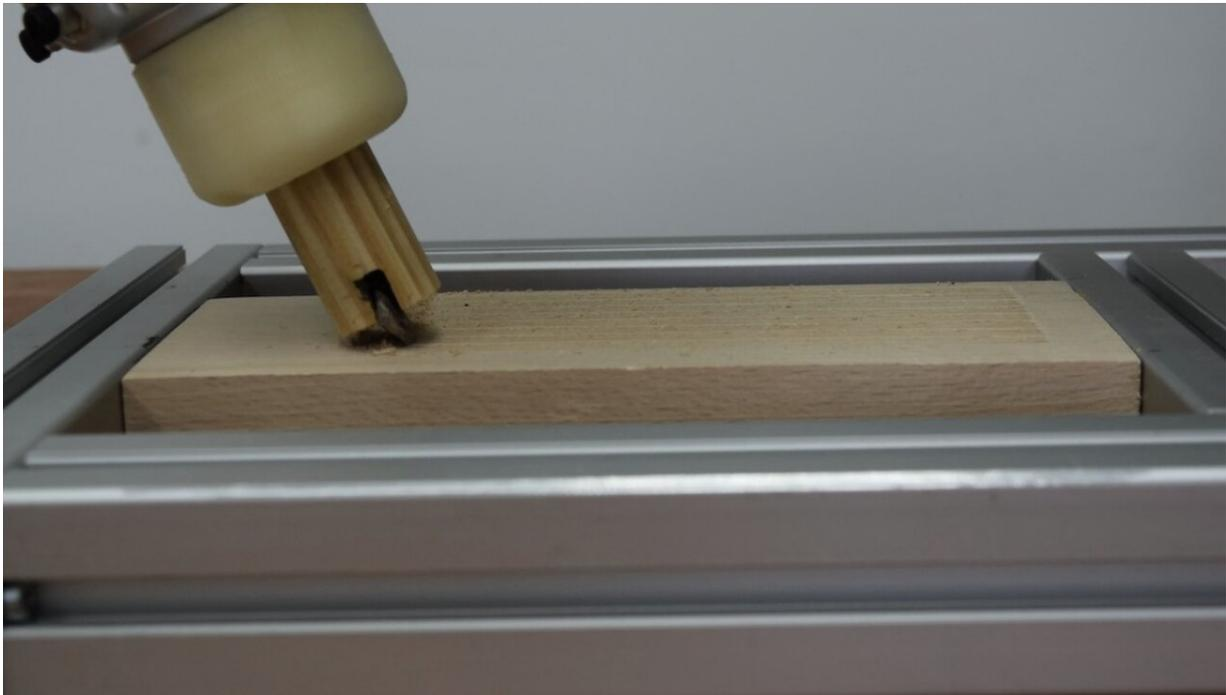
A robot that used force-control technology developed by Ludovic Righetti and Johannes Pfleging tested the adhesive by scraping a block of wood 170 times. Credit: NYU Tandon, Johannes Pfleging
