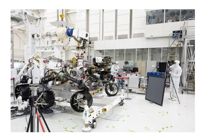
In this image, engineers test cameras on the top of the Mars 2020 rover's mast and front chassis. The image was taken on July 23, 2019, in the Spacecraft Assembly Facility's High Bay 1 at NASA's Jet Propulsion Laboratory in Pasadena, California. Credit: NASA/JPL-Caltech
