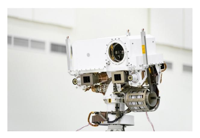
This image, taken in the Spacecraft Assembly Facility's High Bay 1 at the Jet Propulsion Laboratory in Pasadena, California, on July 23, 2019, shows a close-up of the head of Mars 2020's remote sensing mast. The mast head contains the SuperCam instrument (its lens is in the large circular opening). In the gray boxes beneath mast head are the two Mastcam-Z imagers. On the exterior sides of those imagers are the rover's two navigation cameras. Credit: NASA/JPL-Caltech
