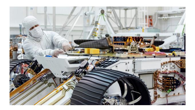
An engineer works on attaching NASA's Mars Helicopter to the belly of the Mars 2020 rover—which has been flipped over for that purpose—on Aug. 27, 2019, at the Jet Propulsion Laboratory in Pasadena, California. Credit: NASA/JPL-Caltech
