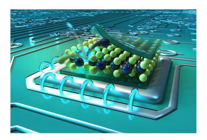
By bombarding thin molybdenum sulfide layers with helium ions, physicists at the Technical University of Munich (TUM) succeeded in placing light sources in atomically thin material layers with an accuracy of just a few nanometers. The new method allows for a multitude of applications in quantum technologies. Credit: Christoph Hohmann / MCQST
