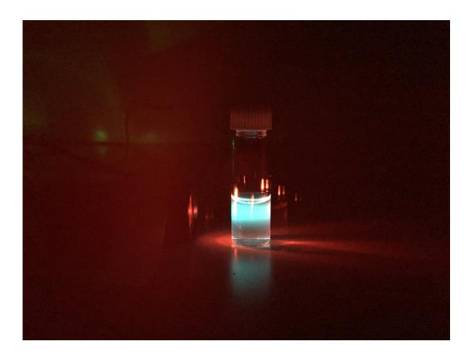
Organic nanoparticles in a vial convert invisible near-infrared light to intense blue light, which can easily be seen by human eyes. Credit: Gang Han
