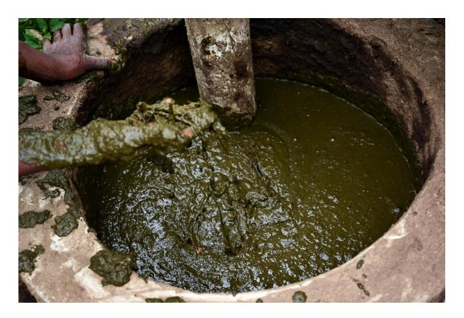
Cow manure has to be mixed with a little water, and twigs have to be sifted, to prevent the biodigester from getting clogged
