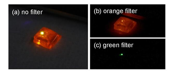
Probing crystals' unique electronic properties by using ODPL spectroscopy. Credit: Kazunobu Kojima, Tohoku University
