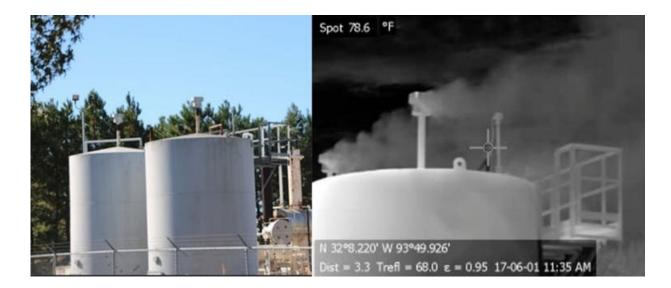
Left: a natural gas storage tank as it would look to the naked eye. Right: the tank as seen by an infrared camera, showing methane gas being vented from the tank, a regular procedure to maintain safe pressure. Credit: Robert Howarth/Biogeosciences, Author provided
