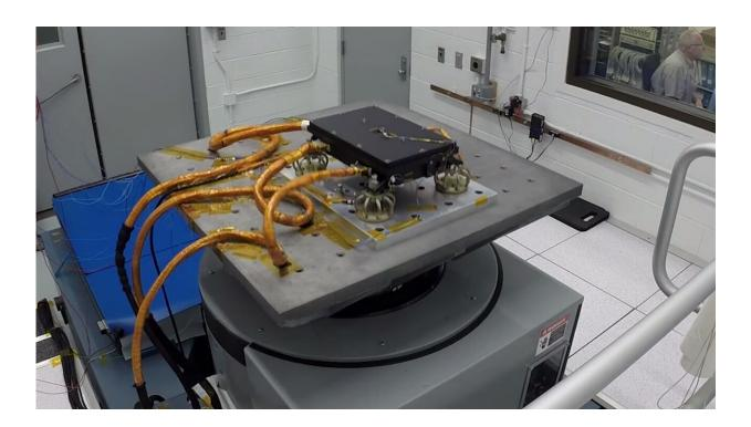
Vibration testing of the MEDLI2 primary electronics box was successfully completed recently at NASA's Langley Research Center in Hampton, Virginia. Flight hardware is being shipped and installed on the Mars 2020 entry vehicle in preparation for next year's launch. Credit: NASA
