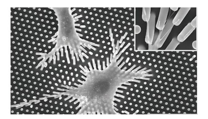
Elastic polydimethylsiloxane (PDMS) micropillars seeded with vascular muscle cells let researchers quantify cellular force and energy during allostasis. Credit: NYU
