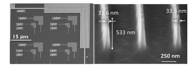
Left: A scanning electron microscope (SEM) image of silicon elbow-shaped nanopatterns with different feature sizes (linewidths). Right: A highmagnification SEM image of high-resolution, high-aspect-ratio silicon nanostructures patterned at a pitch resolution (linewidth plus spacewidth, or space between lines) of 500 nm. Credit: Brookhaven National Laboratory
