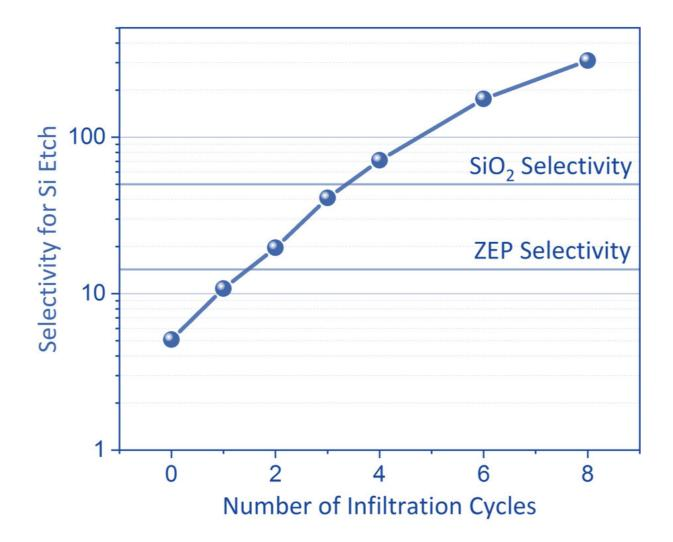
After two processing cycles, the etch selectivity of the hybrid resist surpasses that of ZEP, a costly resist. After four cycles, the hybrid resist has a 40 percent higher etch selectivity than that of silicon dioxide ( $SiO_2$ ). Credit: Brookhaven
