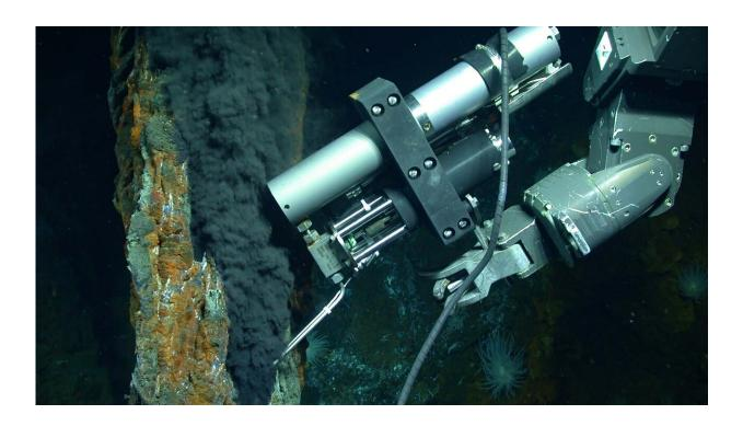
The manipulator arm of the remotely operated vehicle Jason samples a stream of fluid from a hydrothermal vent. The fluid contains gases that are in liquid form because of the high pressure of the deep ocean. Credit: Chris German/WHOI/NSF, NASA/ROV Jason 2012, © Woods Hole Oceanographic Institution
