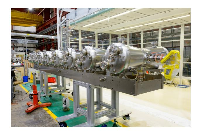
Scientists and engineers at Argonne led the design of these eight accelerator cavities, of a type called half-wave resonators, for the PIP-II accelerator. The Argonne team worked with Fermilab in the design. Credit: Argonne National Laboratory. Fermi National Accelerator Laboratory
