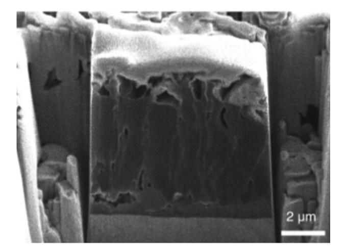
SEM image of the cross section of a columnar microstructure, which leads to high Coulombic efficiency. Credit: Meng lab/Nature
