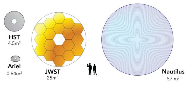
While this is not what the Nautilus mirrors will look like, this illustration shows the total collecting power of the fleet of 35 space telescopes. Each individual Nautilus mirror will, however, be able to collect more light than the Hubble Space Telescope. Credit: Nautilus team
