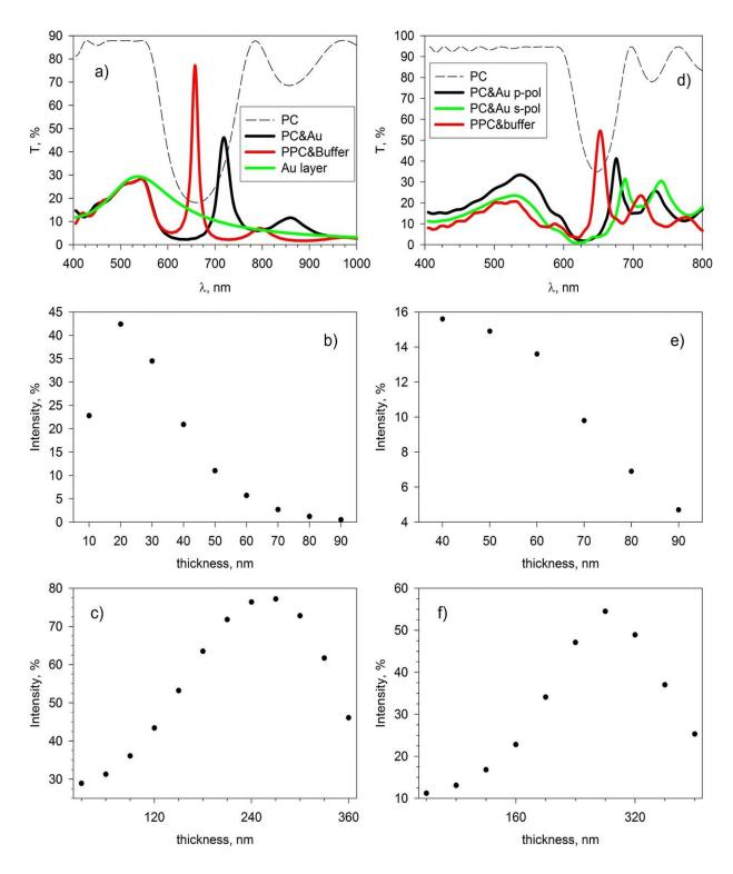
a) Transmission spectra of 1D PC and PPC. Dashed line is the spectrum of PC. Thick line is the spectrum of PC with the 30-nm Au layer. Red line is the spectrum of PC with the 30-nm Au and 270-nm buffer layers. The thin line is the calculated transmission spectrum of the 30-nm Au layer. b) Intensity of
