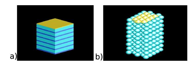
Schemes of PPC with equal effective refractive index and structure period. a 1D PPC and b 3D opal-like PPC. Credit: Kazan Federal University
