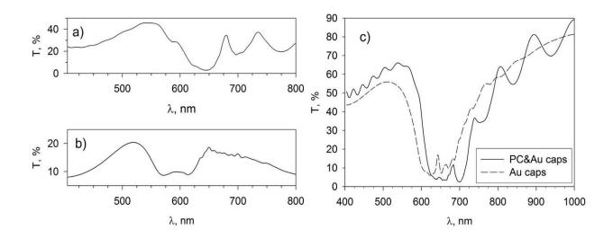
a) Transmission spectrum of PPC with the 30-nm Au layer. b) Transmission
