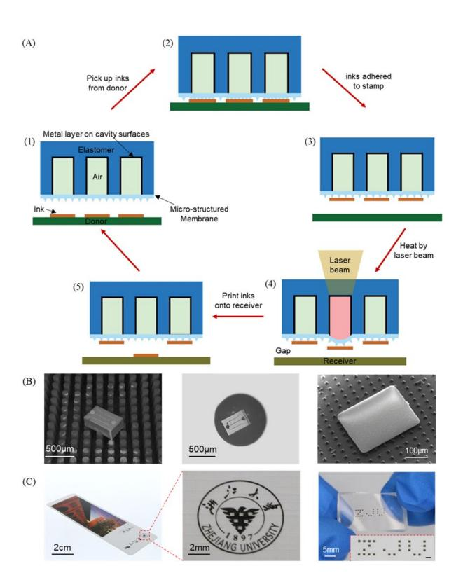
(A) Schematic illustration of the laser-driven programmable non-contact transfer printing process via an active elastomeric micro-structured stamp. (B) Printing
