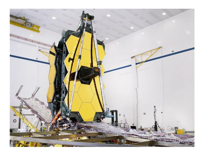
The fully assembled James Webb Space Telescope with its sunshield and unitized pallet structures (UPSs) that fold up around the telescope for launch, are seen partially deployed to an open configuration to enable telescope installation. Credit: NASA/Chris Gunn
