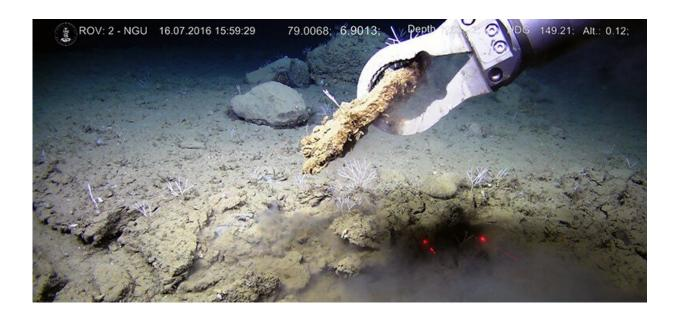
The manipulator arm of the ROV Ægir 6000 samples seep carbonates from the seabed at 1200 m water depth, off western Svalbard. Credit: NORCRUST Using the manipulator arm of the ROV Ægir 6000 aboard R/V G.O. Sars in July 2016 for sampling seep carbonates from the seabed at 1200 m water depth, off western Svalbard. Credit: NORCRUST
