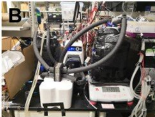
Schematics, images, and control interface of the apparatus for direct contact membrane distillation (DCMD). (A) Schematics of the apparatus for direct contact membrane distillation (DCMD). Visual images of (B) the DCMD reactor and (C) LabVIEW control system
