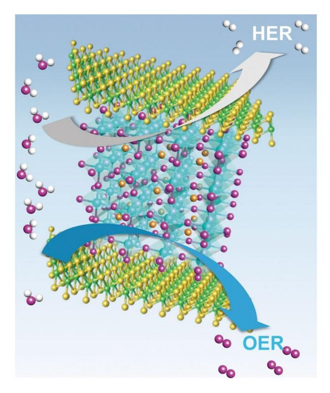
Schematic diagram of proposed charge transfer processes between MoSe<sub>2</sub> and LSC. Credit: UNIST
