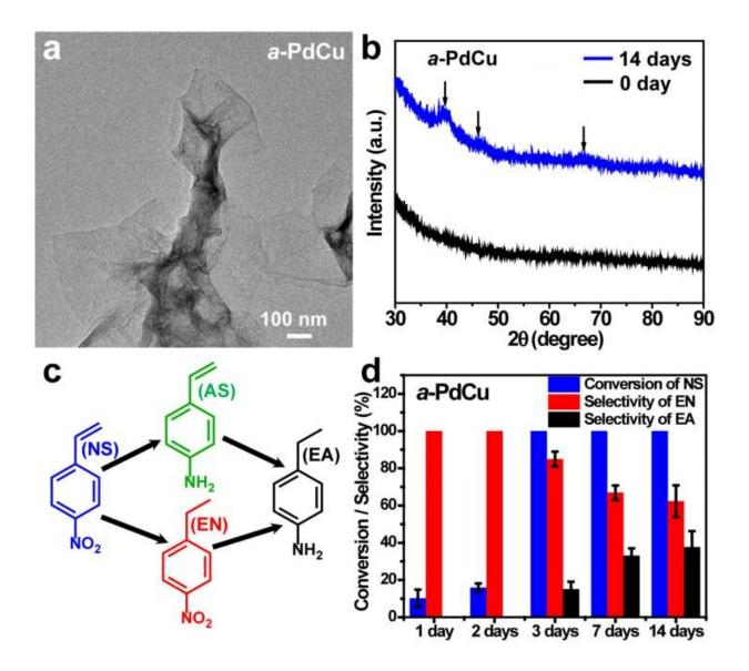
(a) TEM image of a-PdCu nanosheets. (b) XRD patterns of the as-synthesized (0 day) a-PdCu and the a-PdCu after aging for 14 days. (c) Hydrogenation reaction
