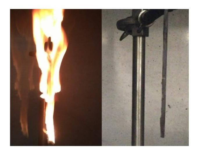
A flammable epoxy resin (left) burns, but one coated with a plant-derived flame retardant (right) does not. Credit: Yoseph Getachew
