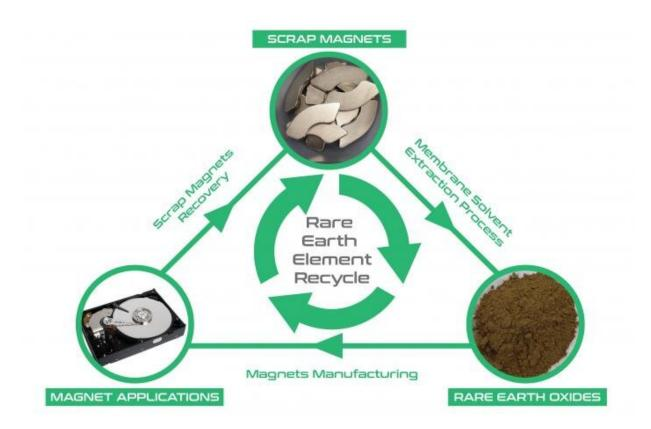
The patented process recovers more than 97% of the rare earth elements from scrapped magnets at purities exceeding 99.5% by weight. The recovered material can be made into new magnets for electronics and other applications. Credit: Oak Ridge National Laboratory, U.S. Dept. of Energy; created by Syed Islam and Jason Smith
