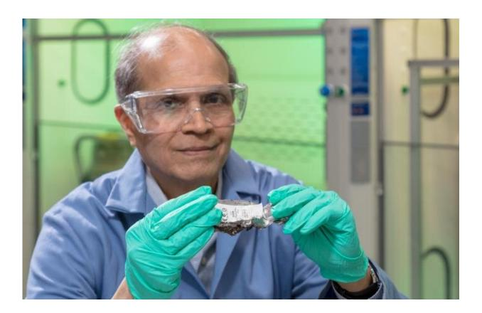
Oak Ridge National Laboratory's Ramesh Bhave co-invented a process to recover high-purity rare earth elements from scrapped magnets of computer hard drives (shown here) and other post-consumer wastes. Credit: Carlos Jones/Oak Ridge National Laboratory, U.S. Dept. of Energy
