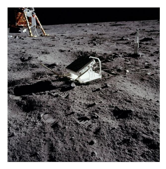
Lunar Laser Ranging Experiment on the surface of the Moon, used by astronomers to calculate the distance to the moon. Credit: NASA
