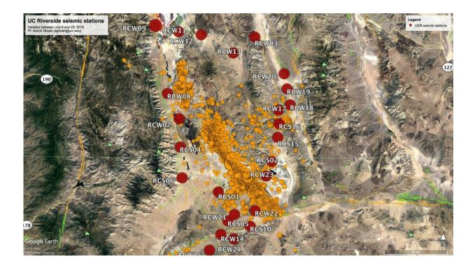
Map of the UC Riverside seismic station network. Red circles indicate location of the stations, yellow circles indicate aftershock location and size. Yellow and green lines are mapped, known fault lines. Credit: UCR
