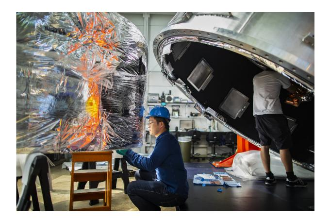
As part of the largest ground-based cosmic microwave background (CMB) experiment ever built, twice as big as previous observatories, putting together the large aperture telescope receiver (right) for the Simons Observatory will be a multiyear endeavor for researchers in Mark Devlin's lab. Credit: University of Pennsylvania
