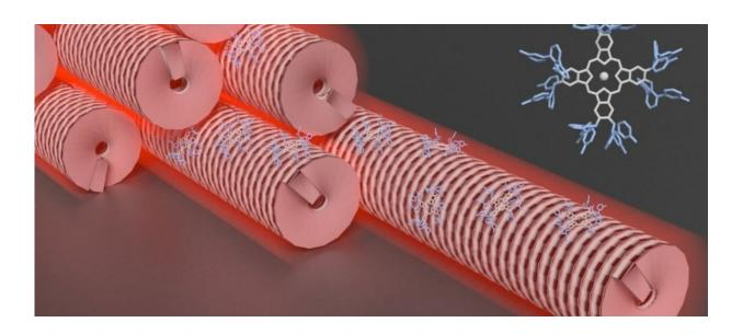
Schematic representation of the photoactive rod-like virus bundles glued together by action of the dye (top-right corner). Credit: Aalto University
