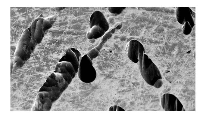
SEM image of corroded nickel at the surface. Credit: Mengying Liu
