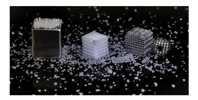
How do you turn salt and magnesium (left) into a bone implant with regularly structured pores (right)? ETH researchers developed a method using a template of 3-D-printed salt (centre). Credit: Laboratory of Metal Physics and Technology / Complex Materials / ETH Zurich
