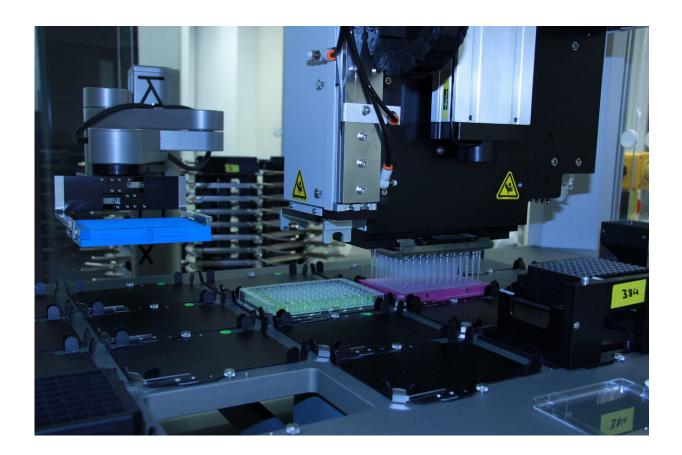
Integrated robotic workstation used at EPFL's Biomolecular Screening Facility for performing combinatorial synthesis of macrocycles and subsequent highthroughput target-based screening assays. Credit: Antoine Gibelin (EPFL)
