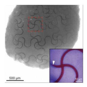
This cyborg organoid is fully integrated with stretchable, mesh nanoelectronics. Credit: Jia Liu/Harvard SEAS)
