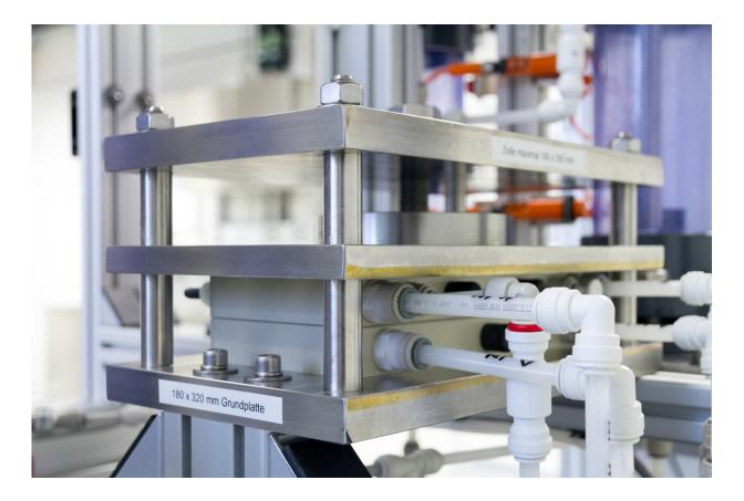
Electrochemical cell for CO2 reduction. Credit: Fraunhofer IGB
