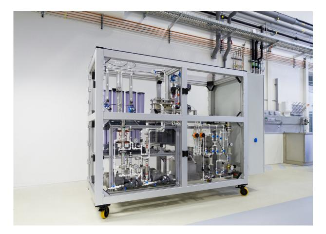
Demonstrator for the one-step electro-chemical production of ethylene from CO2 and water. Credit: Fraunhofer IGB
