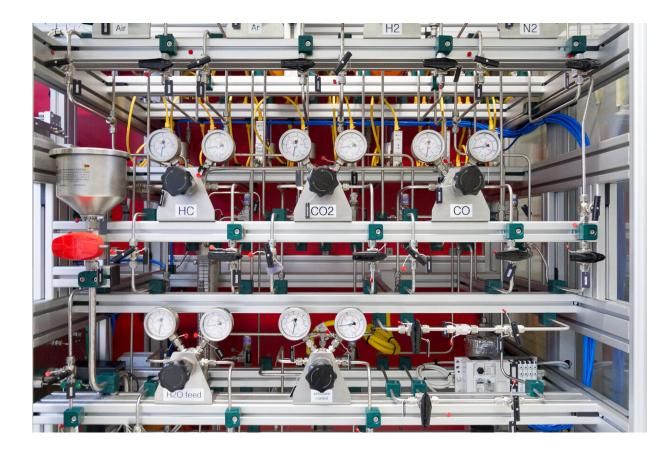
In this multi-purpose system with four parallel reactor tubes, the researchers can test catalysts under different reaction conditions in high throughput. Credit: Fraunhofer-Gesellschaft
