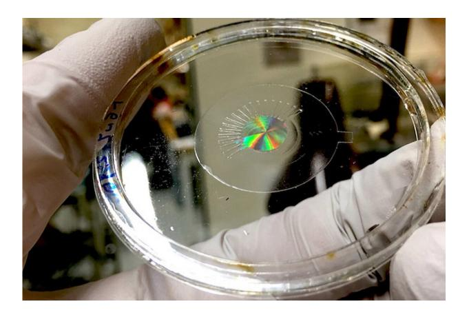
The metalens (made of silicon) are mounted on a transparent, stretchy polymer film, without any electrodes. The iridescence is produced by the large number of nanostructures within the metalens. Credit: Alan She/ Harvard SEAS
