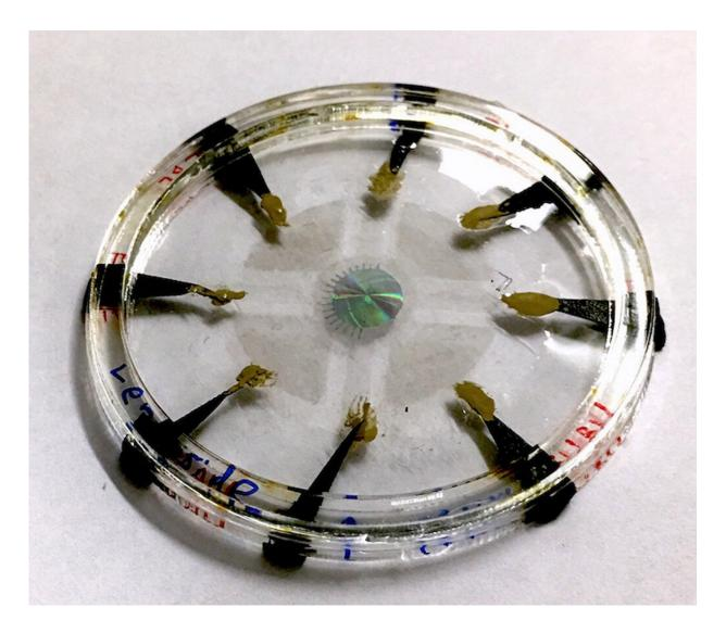
The actual device, in which the adaptive metalens (center) is controlled by embedded electrodes made of carbon nanotubes. Credit: Alan She/ Harvard SEAS
