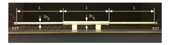
Experimental setup, consisting of a waveguide bar with cavity and side channels. The excitation of elastic waves traveling along the bar is provided by piezoelectric actuators placed at the two ends of the system. Credit: Giuseppe Trainiti, Georgia Tech
