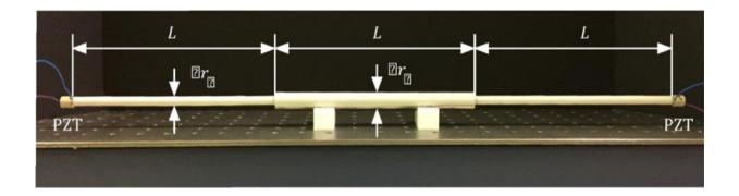
Experimental setup, consisting of a waveguide bar with cavity and side channels. The excitation of elastic waves traveling along the bar is provided by piezoelectric actuators placed at the two ends of the system. Credit: Giuseppe Trainiti, Georgia Tech
