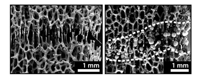
The strut-and-gap internal structure of a metallic foam reduces its weight while maintaining its strength, but makes it impossible to repair with traditional methods, which would melt that structure away. In the new technique, electrochemistry adds new metal just to the broken struts, reconnecting them and "healing" the damage. Credit: Pikul Research Group
