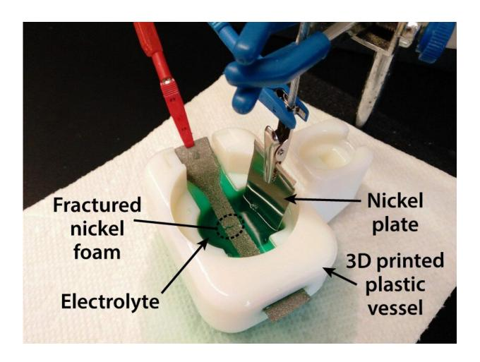
The researchers placed their fractured samples into an electroplating bath. Nickel ions are transported through the open structure within the metal foam, but
