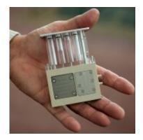
The ESP holds 60 cartridges, each programmed to collect water at specific "sampling events." Credit: MBARI
